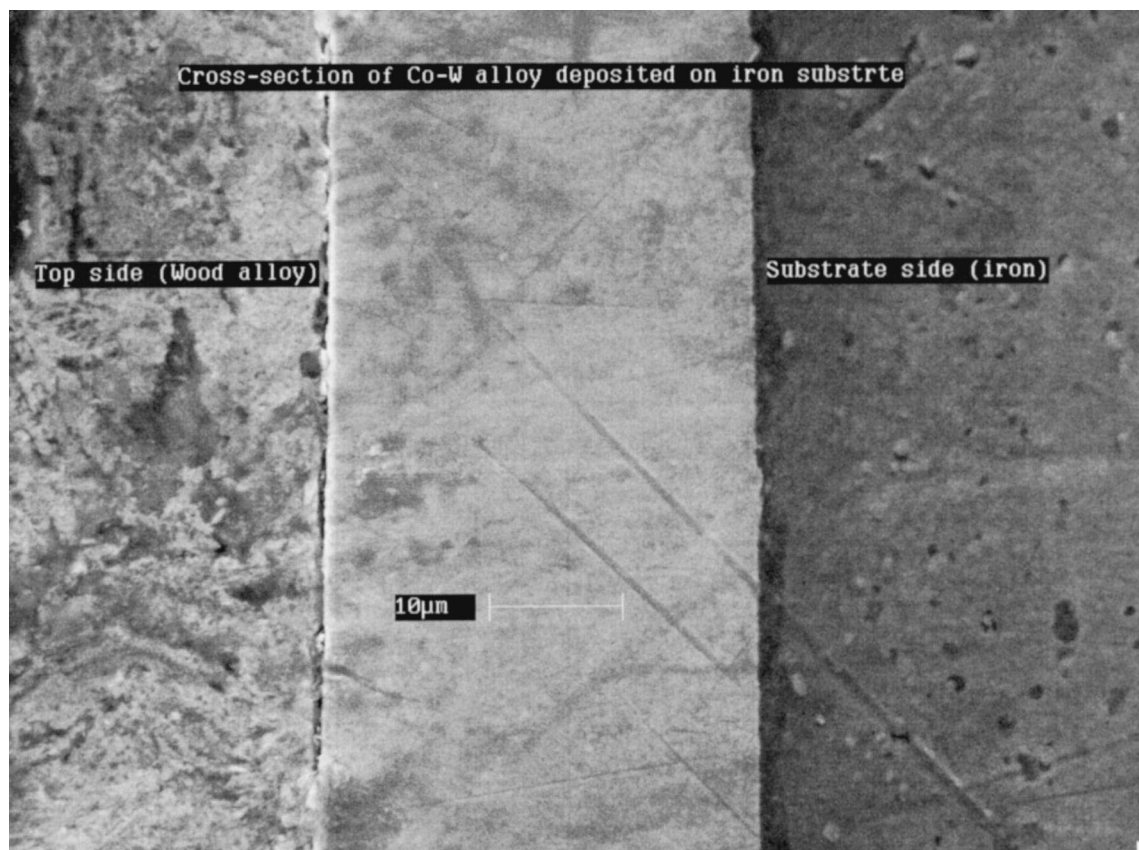
Fig. 4. SEM image of a Co-W amorphous-alloy cross section prepared for EDS/WDS analysis.
